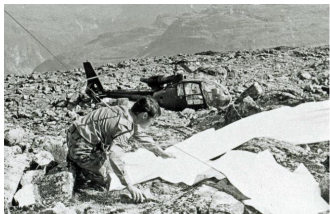
After being helicoptered to a summit Corporal Jimmy Hamilton sets out a pre-mark ready for the spotting photography.
