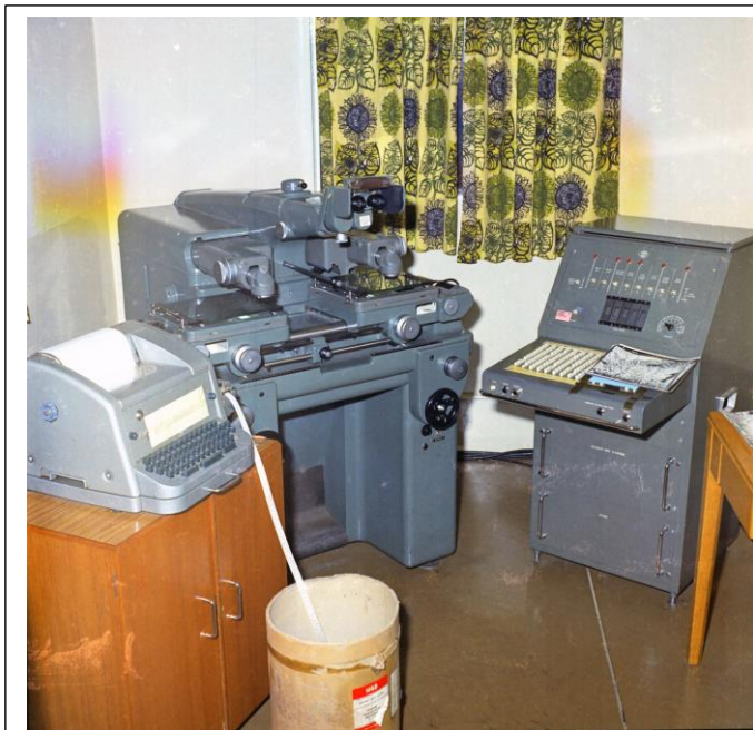
The Kampen sheet was the first task that used Air Survey Troop's Hilger and Watts Stereocomparator in Block 101. Its automatic recording capability and paper tape output were innovative at the time.
